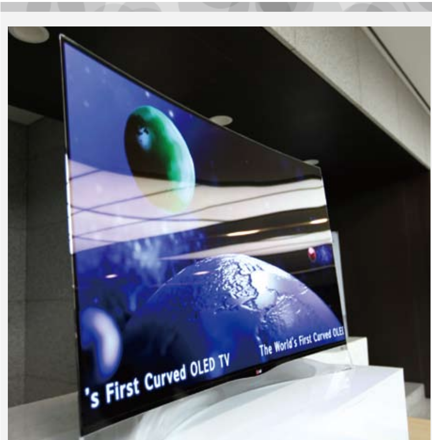
55-inch Curved OLED TV • Application of concave curve to both sides for the first time in the world • Minimized picture distortion, outer section awareness decline by applying the same distance from the viewer's eye to screen center and sides, respectively
